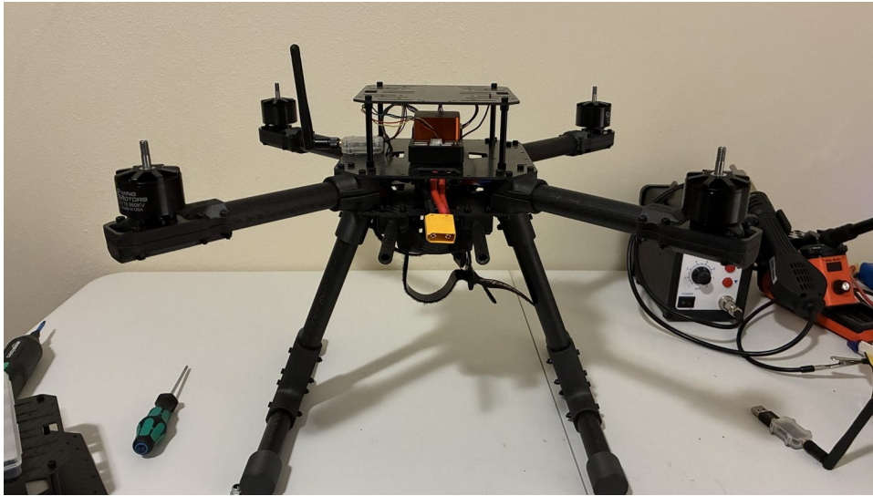
The built airframe before props: compute plate on its standoffs above the flight controller, arms level, legs splayed.
