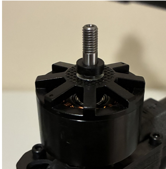
An adapter ring seated on the motor shaft, ready for the prop.
